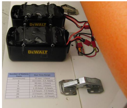
Figure 1.4: Battery Compartment with Hot-swappable Packs
